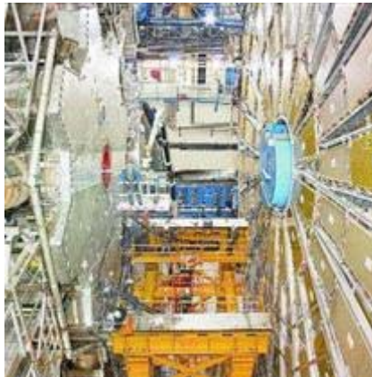
CREDIT: Prof. Robert McPherson, UVic IPP / The ATLAS, a 100-tonne precision particle detector that is nine metres in diameter, has been lowered into place in Switzerland. Vancouver researchers helped design and build the enormous detector.
